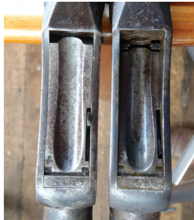
RIGHT: Left, the action closed and cocked – right, the action open with the extractor and chamber visible.
