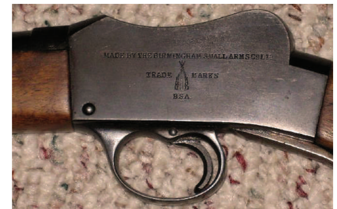
A standard BSA Cadet receiver. Note the head of the pin which is punched out to remove the action and trigger group etc.
