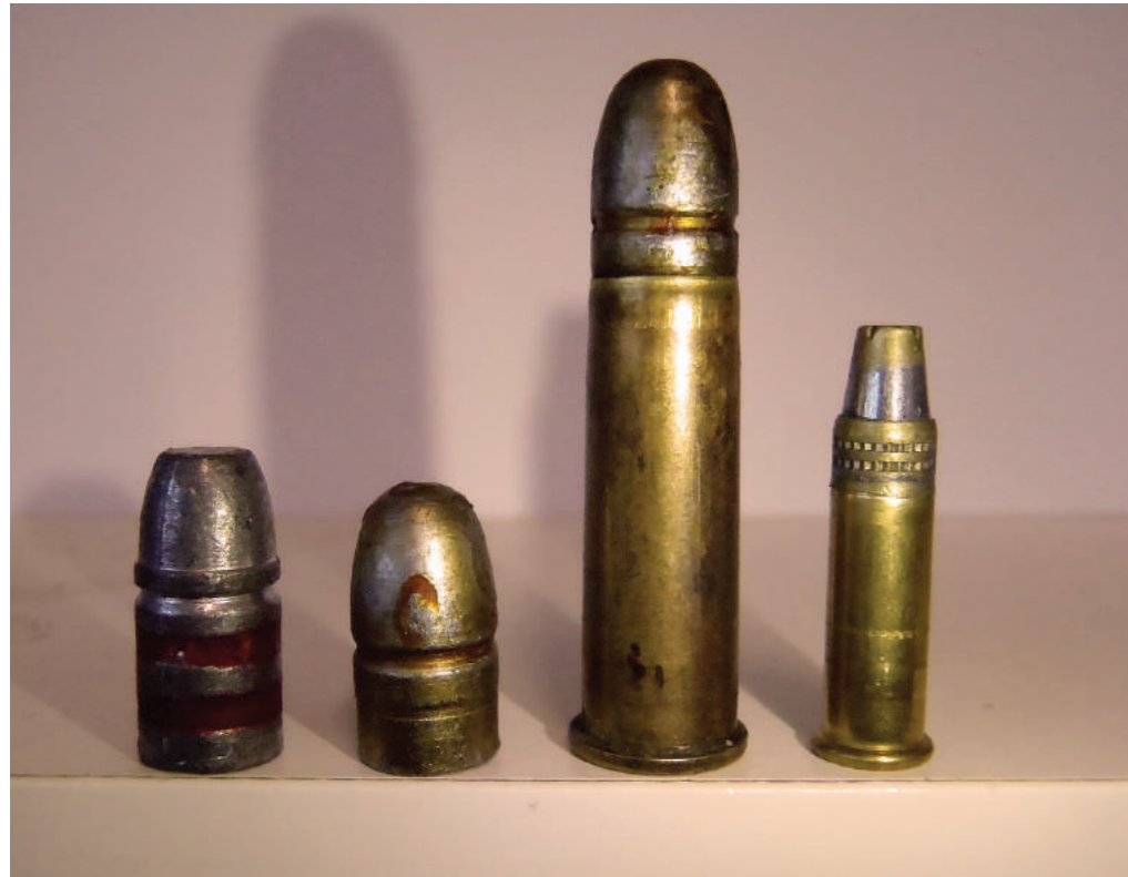
From the left; .316" Taipan 125 grain internally lubricated projectile, CBE 320-120 heeled projectile externally lubricated with Lee Liquid Alox, a loaded round – note that the case is the same outer diameter as the projectile, and right, a .22lr which is also externally lubricated with a heeled projectile.
