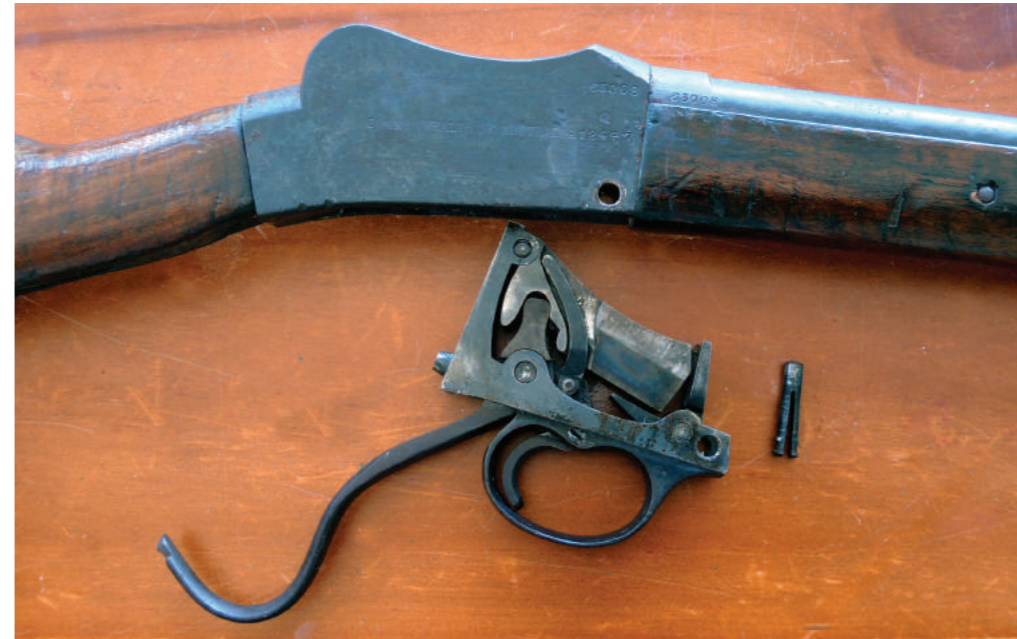
With the single split pin tapped out (right) the Cadet's internal components can be removed for cleaning and maintenance.
