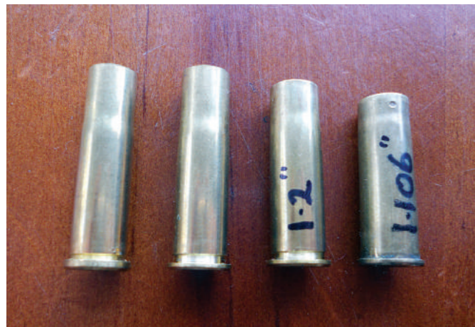
From the left: New Winchester .32/20 case, .32/20 case with rim trimmed to .044", case trimmed to 1.2" sized and fire-formed, factory Kynoch .310 case for comparison.
