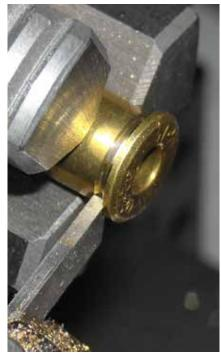
The thickness of a .32-20 case rim is best reduced by removing brass from the front of rim, not the rear (see text).
