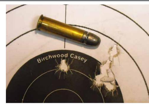
A 50 metre group shot with the cast CBE 325 125 bullets and a duplex load comprising a layer of AR2205 behind Swiss blackpowder.
