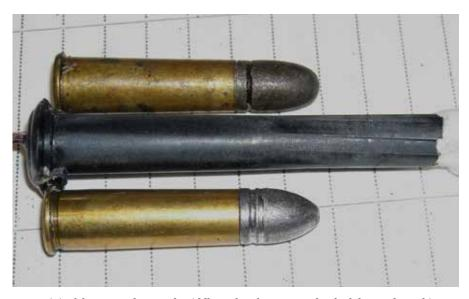
Top; original factory Cadet round, middle; a chamber cast made of sulphur and graphite powder, bottom; a short case with one of Jeff's cast CBE 325 125 bullets.
