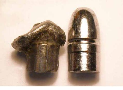
Left; a CBE 320 120 bullet cast in 40-1 alloy recovered from wet phone books at 50 metres. Upon firing the heel has slugged up to groove diameter and there's still some lube left in the groove.
