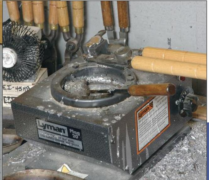
*Left, Mike's casting area includes an exhaust fan and a small manicurist's fan (to his left) for cooling sprues. Above, bullet moulds are preheated atop the lead furnace. The same goes for the ladle.*
