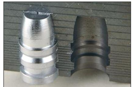
*Above, when a mould does not close properly, there will be flashing all around the freshly poured bullet. Below, the mould pin alignment hole on the right can be seen to be slightly peened. That mould is not going to close properly and drop its best bullets until fixed.*
