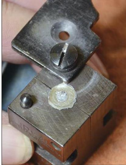
*When flashing forms atop a bullet mould, it is a sign of a too-loose sprue plate.*
