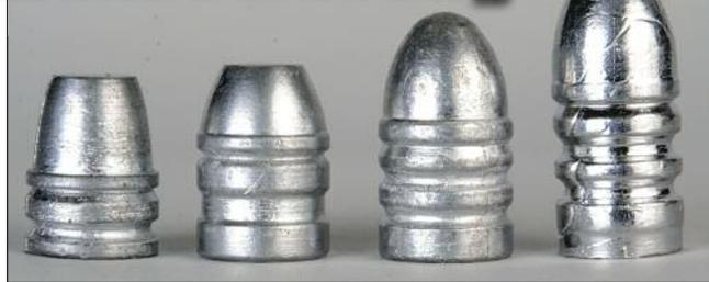
*The bullet at far right is simply the result of the mould and/or alloy being too cool. Conversely, the three bullets at left have been poured with a contaminated alloy that does not allow bands and edges to fill out perfectly.*
