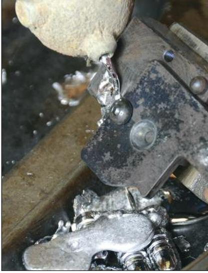
*Above, to remove lead smears from atop a set of mould blocks, Mike ladles molten alloy on it until the smear turns shiny. Then it too is molten and can be rubbed off with a piece of cloth. Right, perhaps the most common problem besetting bullet casters is lead smears across the top of moulds. They must be removed for a bullet's base to be perfectly flat.*
