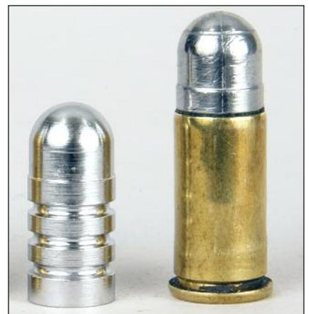
*The Lyman 358430 bullet (left) is perfectly formed. The loaded bullet in .38 S&W (right) has some minor wrinkles in its nose that will not be a detriment to accuracy.*
