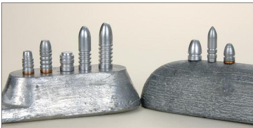
Mike uses only 1-to-20 (tin-to-lead) foundry alloy for revolver bullets and BPCR bullets (left). For modern rifle bullets and autoloading pistol bullets (right), he uses only Linotype.
